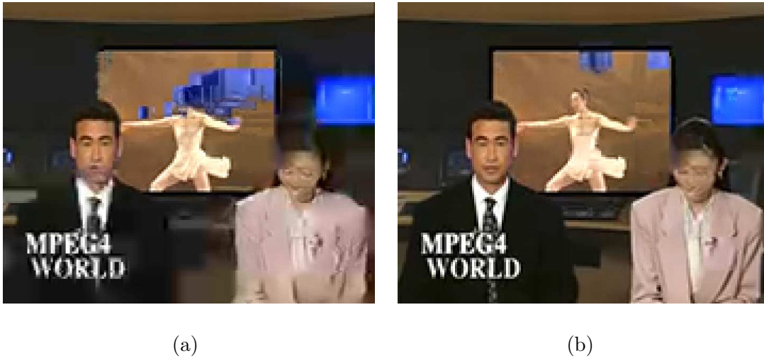
Fig. 6. Frame 33 (100 in original) News QPB:45 QPE:25, EEP, BER = 10e-3, (a) Upward, (b) Proposed.
